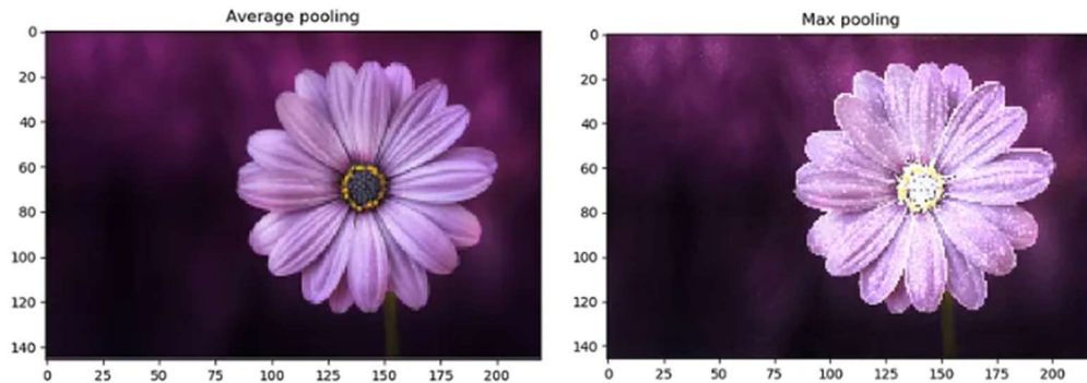
Figura 3 –Max Pooling e Average Pooling
